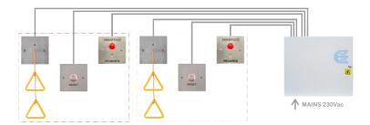
For example, consider a local system comprising 2-off toilets, e.g. Ladies and Gents, each with pull cords, beacon/sounders and reset units. A single PSU-NIOSPro-SVR2 could be used to provide two independent alarm zone controllers in a single wall mount enclosure. In this case, each alarm could be activated independently; and the monitoring equipment would report which of the two alarms have been activated.
