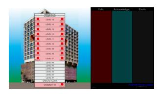
The upgraded version of our reliable NIOS workstation offering a user-friendly plan-based GUI, indicating the source of alarms. This workstation can be supplied in desk, wall mount and touch-screen formats to suit site and operational requirements.
