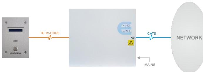
A typical application is to connect a remote LCD indicator panel to a network. To display alarms and faults reported by other network devices.
