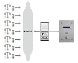
Document M compatible alarm monitoring with acknowledge function for up to 8 alarms
