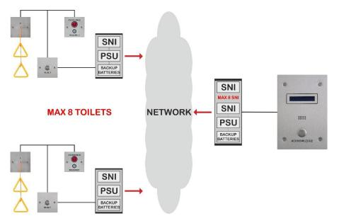
Document M compatible alarm monitoring with acknowledge function for up to 8 alarms
