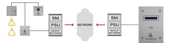
Document M compatible alarm monitoring with acknowledge function for single alarm
